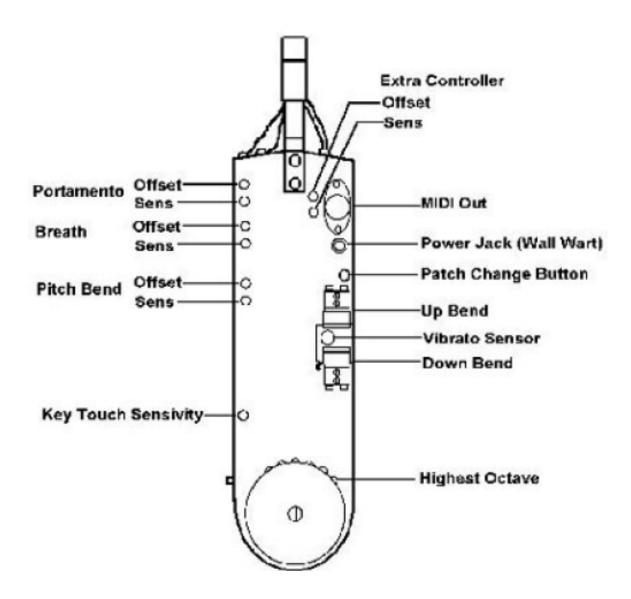
Note: The "extra" controller is in the mouthpiece post, which is made of aluminum. It is touch sensitive and is connected to a lip controller that adds Foot Control midi when you increase contact with your skin.
